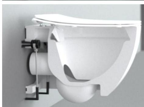
Fit the plastic handle to the long hex key and use this to tighten the hex screws in the plastic fittings. If this pan is being fitted to a tiled wall, it is advisable to apply a bead of silicone between the rear of the pan and the tiles. This is to prevent the tiles cracking as the pan is tightened to the wall.
