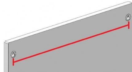
Hang the mirror onto the wall fixings, ensuring that they are located securely into the inserts.
