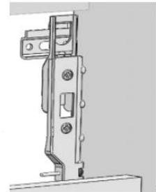
A securing screw should be fitted through the back of the unit through the fixed back of the cabinet and into the wall, this will help to stabilise the unit.
