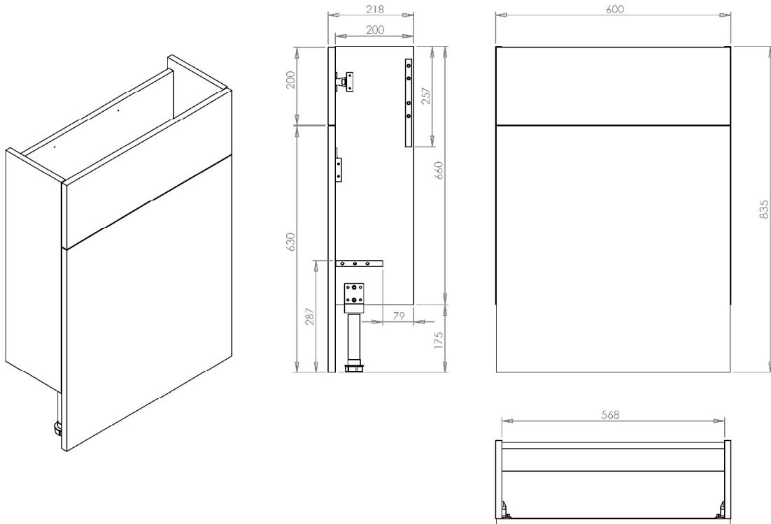
All dimension in mm. Please check dimensions prior to installation as they can vary due to manufacturing tolerances.
