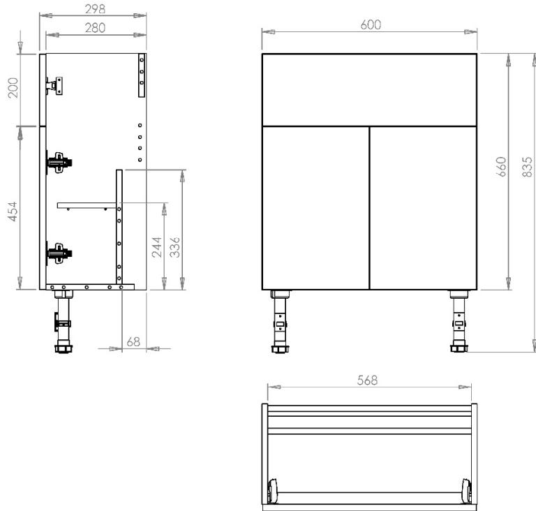
All dimension in mm. Please check dimensions prior to installation as they can vary due to manufacturing tolerances.
