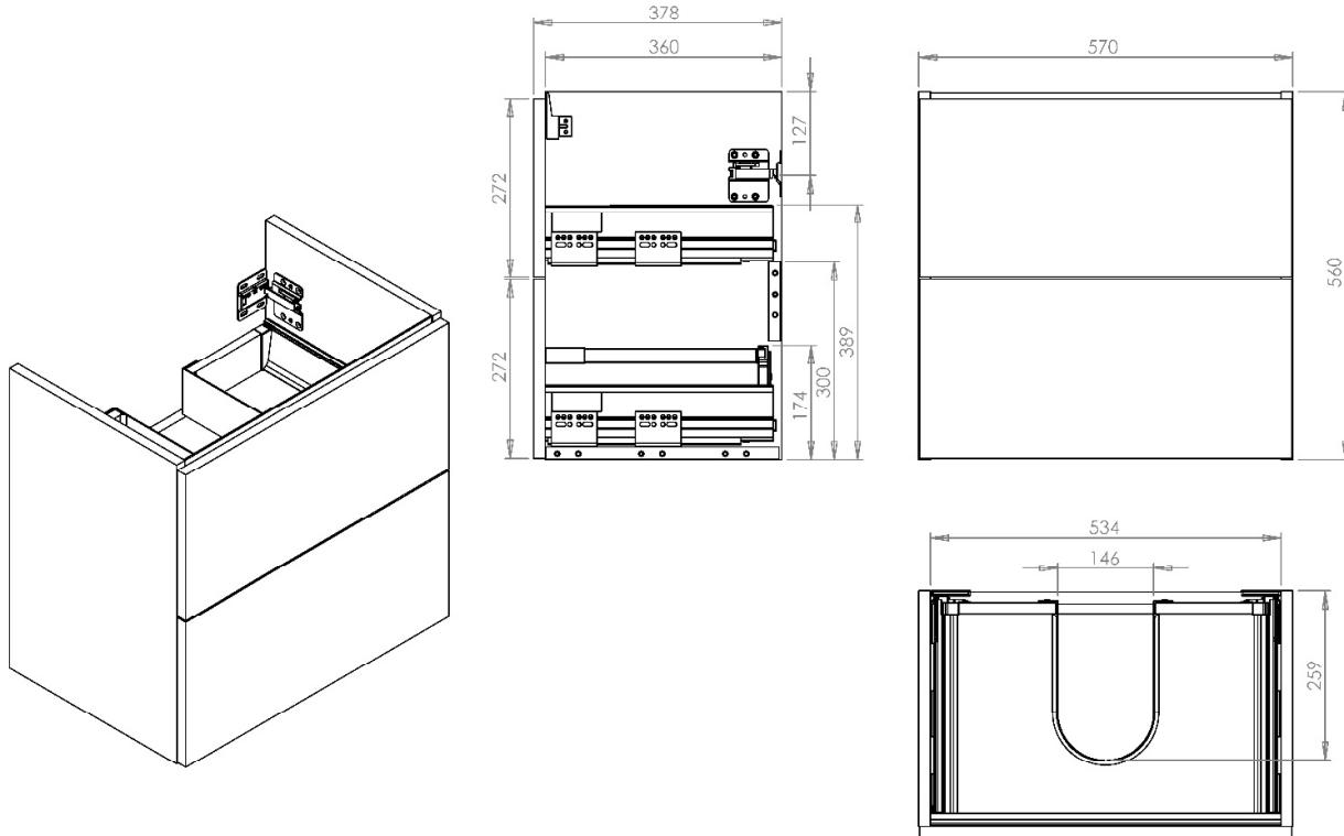
All dimension in mm. Please check dimensions prior to installation as they can vary due to manufacturing tolerances.
