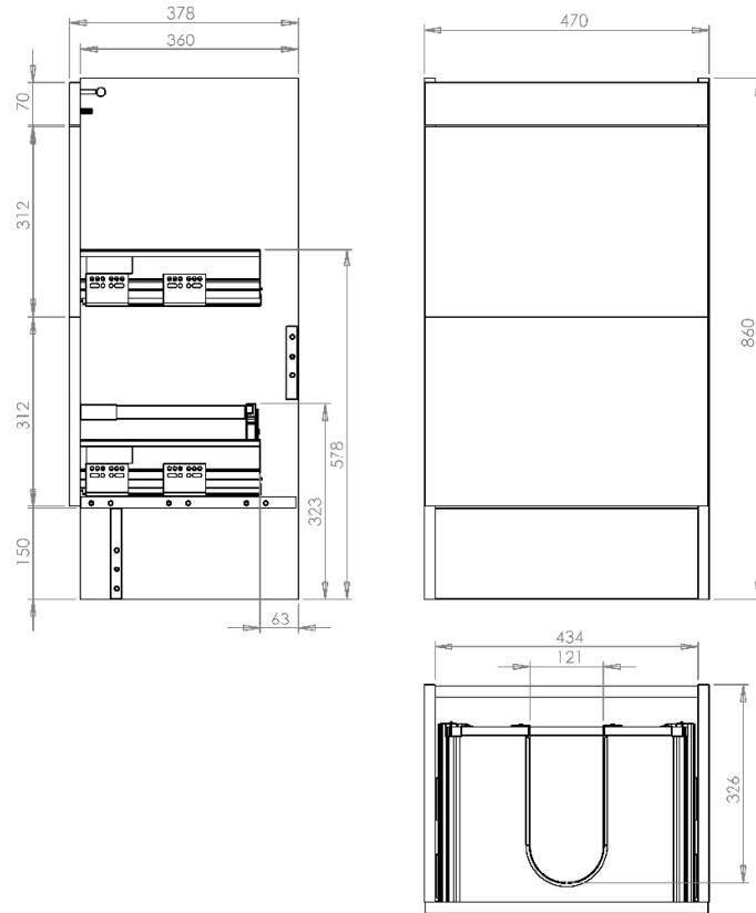
All dimension in mm. Please check dimensions prior to installation as they can vary due to manufacturing tolerances.
