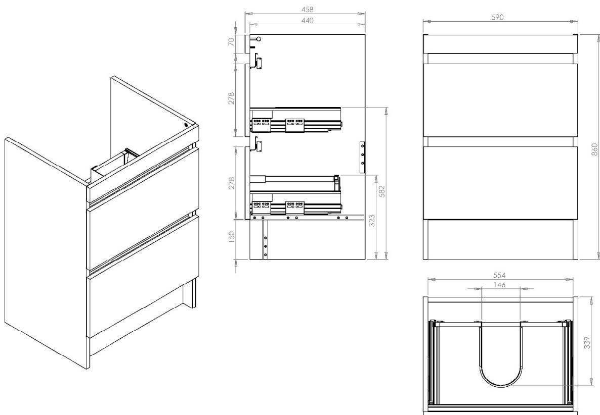
All dimension in mm. Please check dimensions prior to installation as they can vary due to manufacturing tolerances.
