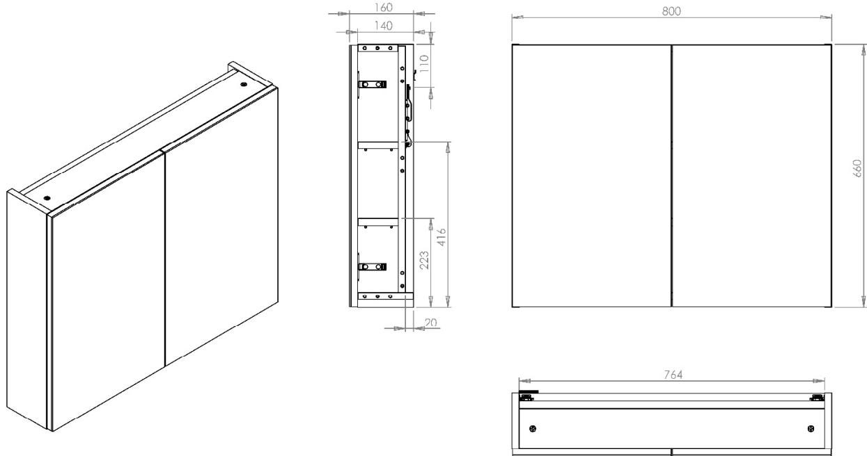
All dimension in mm. Please check dimensions prior to installation as they can vary due to manufacturing tolerances.
