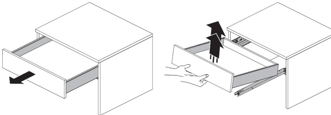
Remove the cover cap strips from the top of the drawer box sides by carefully pulling them upwards.
