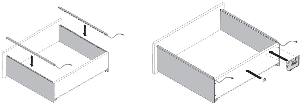
Screw the battery pack in its holder onto the rear of the drawer box. The battery pack must be fitted flush to the top of the drawer box and as far over to the right of the drawer box as possible. A spacer is included if it is required to move the battery box further away from the drawer back.
