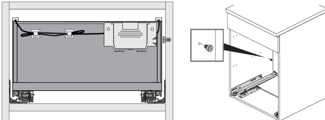
Fit the drawer box back into the cabinet. Pull the drawer runners out to their full extension. Place the drawer box on to the drawer runners. Push the drawer closed, open it and close it again until you hear the drawer box click into position.
