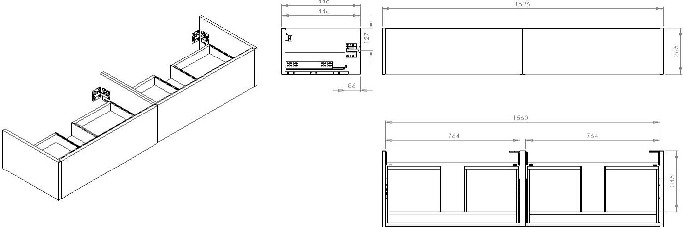
All dimension in mm. Please check dimensions prior to installation as they can vary due to manufacturing tolerances.
