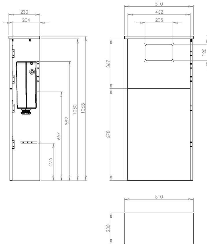
All dimension in mm. Please check dimensions prior to installation as they can vary due to manufacturing tolerances.
