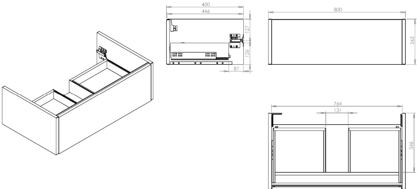
All dimension in mm. Please check dimensions prior to installation as they can vary due to manufacturing tolerances.
