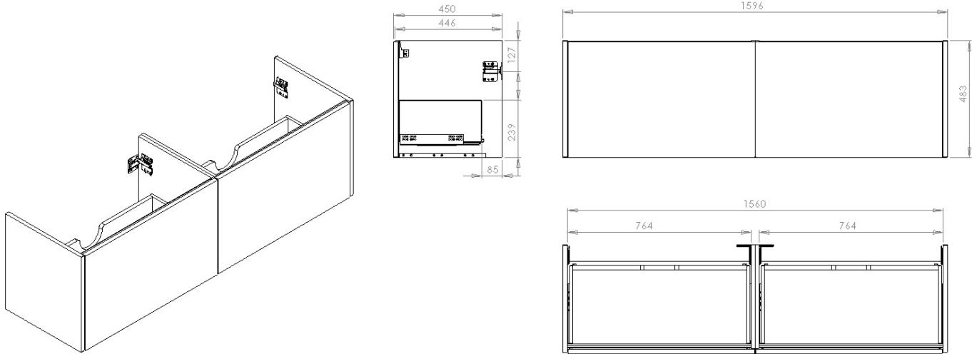
All dimension in mm. Please check dimensions prior to installation as they can vary due to manufacturing tolerances.
