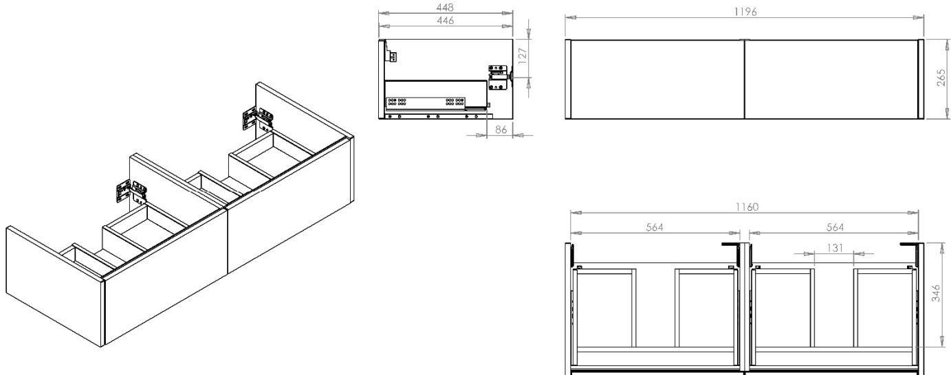
All dimension in mm. Please check dimensions prior to installation as they can vary due to manufacturing tolerances.
