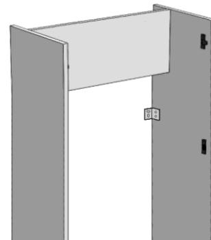
Mark the position of the holes in the stretcher plates on the wall with a pencil. Drill the positions marked with a suitable drill bit.
