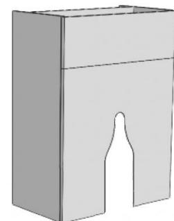
To cut the lower fascia panel to accommodate the soil pipe and cistern flush pipe, use a jigsaw with a fine-toothed blade suitable for timber. Ensure that the room is well ventilated when cutting the material.
