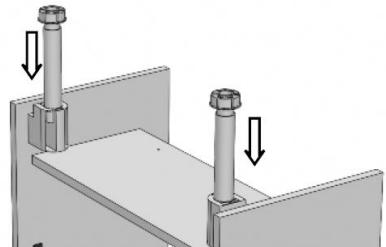
To secure the WC unit against the wall, screw the stretcher plates to the gable panels of the cabinet as shown in the diagram. Ensure that the screws used are suitable for the thickness of the cabinet.
