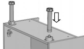
Stand the unit back on its legs against the wall. If fitting a run of units, fix them together through the gable panels. Where possible, try to hide the fixings behind shelves or hinge plates.
