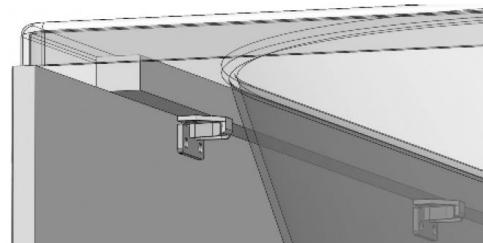
Screw three black Keku clips to the underside of the wooden batten underneath the bath rim using the screws provided. The three clips should be equally spaced along the length of the bath. Use the diagram as a guide to how the Keku clips are fitted.
