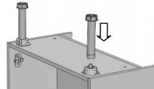
Stand the unit on its legs against the wall. Adjust the legs on the unit until it is level.
