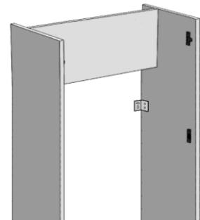
Fasten the unit in position through the stretcher plates using fixings suitable for the wall type.
