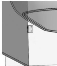
If the bath panel is being used in conjunction with an end panel, secure one "L" bracket to the wall to prevent the panel from being pushed inwards. On the opposite side to the wall, secure the bath panel in place using a Keku clip. This Keku clip is supplied with the end panel, along with instruction on how it is fitted.
