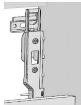
To adjust the position of the cabinet on the wall, use the two screws in each hanging bracket. The top screws will move the cabinet closer to or further away from the wall. The lower screws will move the cabinet up and down.
