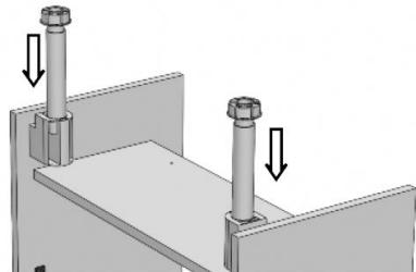
If fitting a run of units, fix them together through the gable panels. Where possible, try to hide the fixings behind shelves or hinge plates.
