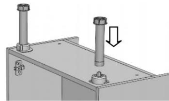
Stand the unit back on its legs against the wall. If fitting a run of units, fix them together through the gable panels. Where possible, try to hide the fixings behind shelves or hinge plates.
