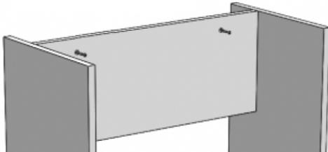
If the unit is to be fitted pulled forward so that it is in line with a run of furniture, secure it in position by screwing into the adjacent cabinet and wall through the gable panels. Try to hide the fixings where possible behind shelves or hinge plates.
