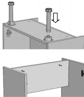
Stand the unit back on its legs against the wall. If fitting a run of units, fix them together through the gable panels. Try to hide the fixings where possible behind shelves or hinge plates.
