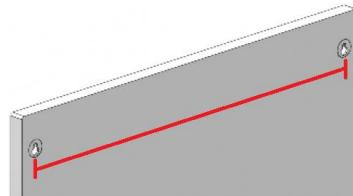
Drill the wall and secure the fixings (not supplied) at the marked positions.
