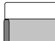
Secure one "L" bracket to the wall using suitable fixings. It is recommended that the bracket is fitted 300mm vertically from the underside of the bath.
