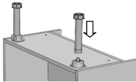
Stand the unit on its legs against the wall. Adjust the legs on the units until they are level.
