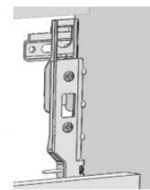
To alter the position of the cabinet on the wall, adjust the two screws in each hanging bracket. The top screws will move the cabinet closer to or further away from the wall. The lower screws will move the cabinet up and down.
