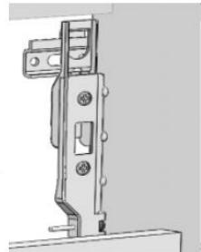
To alter the position of the cabinet on the wall, adjust the two screws in each hanging bracket. The top screws will move the cabinet closer to or further away from the wall. The lower screws will move the cabinet up and down.
