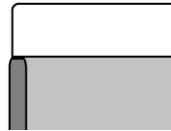
Ensure that when the brackets and bath panel are fitted, the panel sits 4mm proud of the bath rim.
