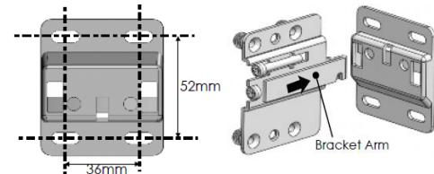
Hook the unit onto the wall brackets so that the spring locks the arm into place.
