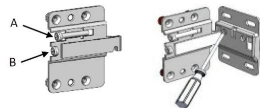
To alter the position of the cabinet on the wall, adjust the two screws in each hanging bracket. Adjusting screws A will move the cabinet up and down. When the cabinet is level on the wall, screws B will tighten the cabinet to the wall.
