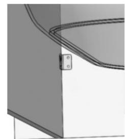
If the bath panel is being fitted between two walls, the two "L" brackets should be secured to the walls to prevent the panel from being pushed inwards. Ensure suitable fixings are used.
