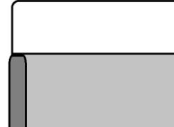
Ensure that when the brackets and bath panel are fitted, the panel sits 4mm proud of the bath rim.
