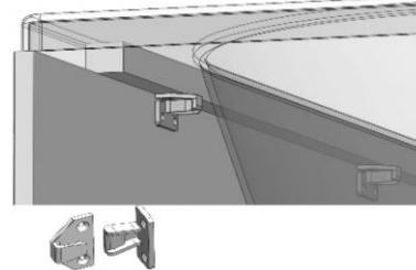
Screw three black Keku clips to the underside of the wooden batten underneath the bath rim using the screws provided. The three clips should be equally spaced along the length of the bath. Use the diagram as a guide to how the Keku clips are fitted.
