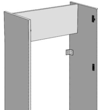
Mark the position of the holes in the stretcher plates on the wall with a pencil. Drill the positions marked with a suitable drill bit.
