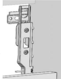
A securing screw should be fitted through the back of the unit through the fixed back rail of the cabinet and into the wall. This will help to stabilise the unit.
