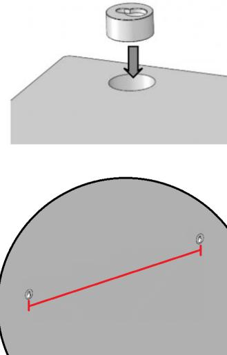
Drill the wall and secure the fixings at the marked positions. Plasterboard or stud walls may require specialist fixings (not supplied). **Note:** you must ensure that the fixings are suitable for the weight of the mirror and the wall type.
