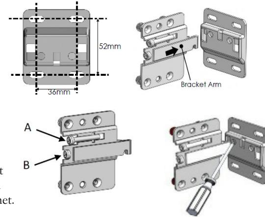
To alter the position of the cabinet on the wall, adjust the two screws in each hanging bracket. Adjusting screws A will move the cabinet up and down. When the cabinet is level on the wall, screws B will tighten the cabinet to the wall.
