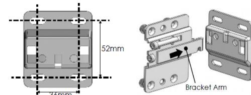
Mark a horizontal line on the wall at the required height **X---X**. Ensure that the wall brackets will fit inside the width of the cabinet and are equally spaced to ensure even distribution of weight. Secure the wall brackets to the wall using suitable fixings. Hook the unit onto the wall brackets so that the spring locks the arm into place.
