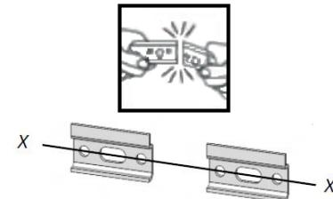
Hook the unit onto the wall brackets ensuring that the brackets are securely located.
