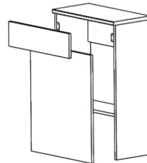
To secure the WC unit against the wall, drill through the rear top rail. Fix the unit in position using suitable fixings.
