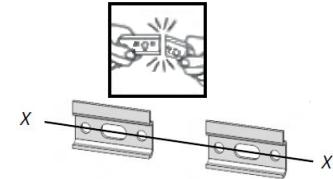
Hook the unit onto the wall brackets ensuring that the brackets are securely located.
