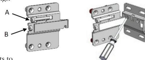
To alter the position of the cabinet on the wall, adjust the two screws in each hanging bracket. Adjusting screws A will move the cabinet up and down. When the cabinet is level on the wall, screws B will tighten the cabinet to the wall.
