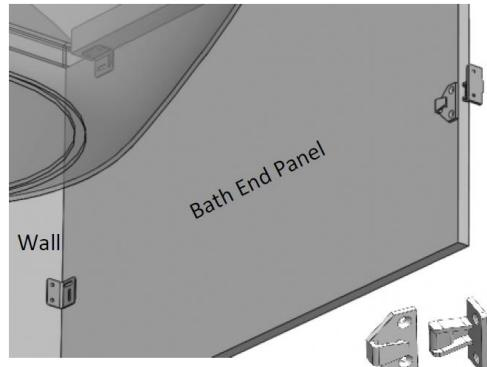
Once fully installed, seal around the bath panel on all joints using a good quality, sanitary-grade silicone sealant.
