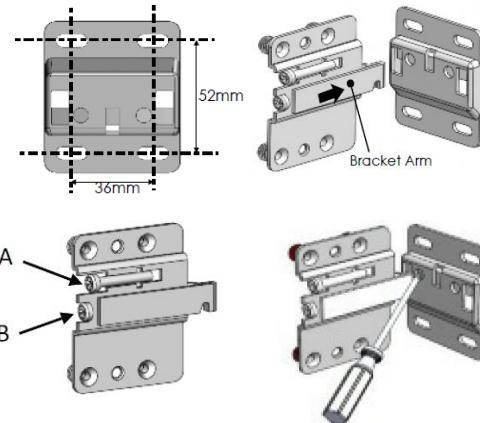
Hook the unit onto the wall brackets so that the spring locks the arm into place.
