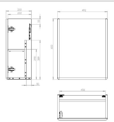
All dimension in mm. Please check dimensions prior to installation as they can vary due to manufacturing tolerances.
