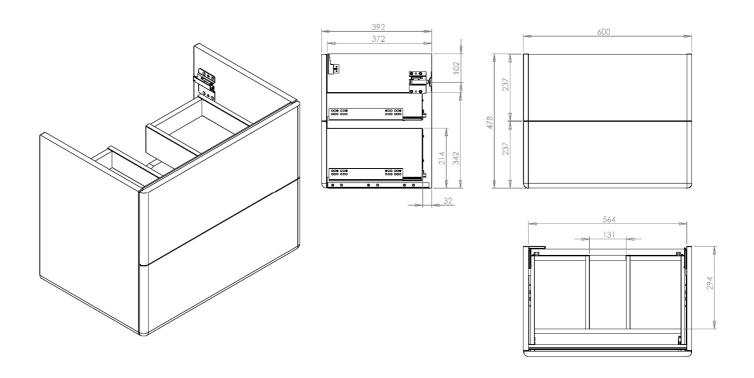
All dimension in mm. Please check dimensions prior to installation as they can vary due to manufacturing tolerances.
