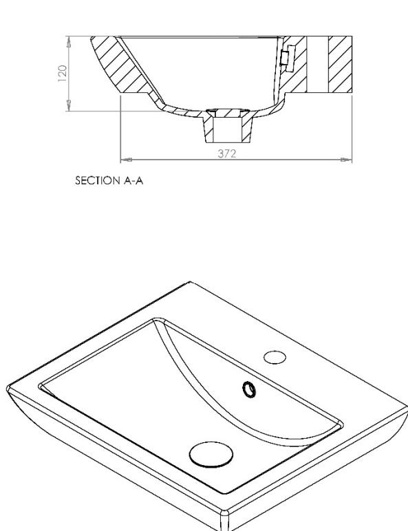
All dimension in mm. Please check dimensions prior to installation as they can vary due to manufacturing tolerances.
