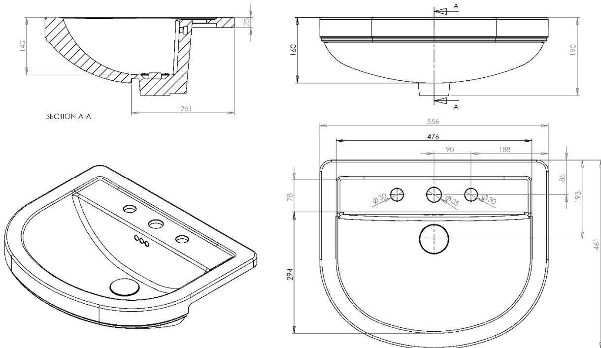
All dimension in mm. Please check dimensions prior to installation as they can vary due to manufacturing tolerances.
