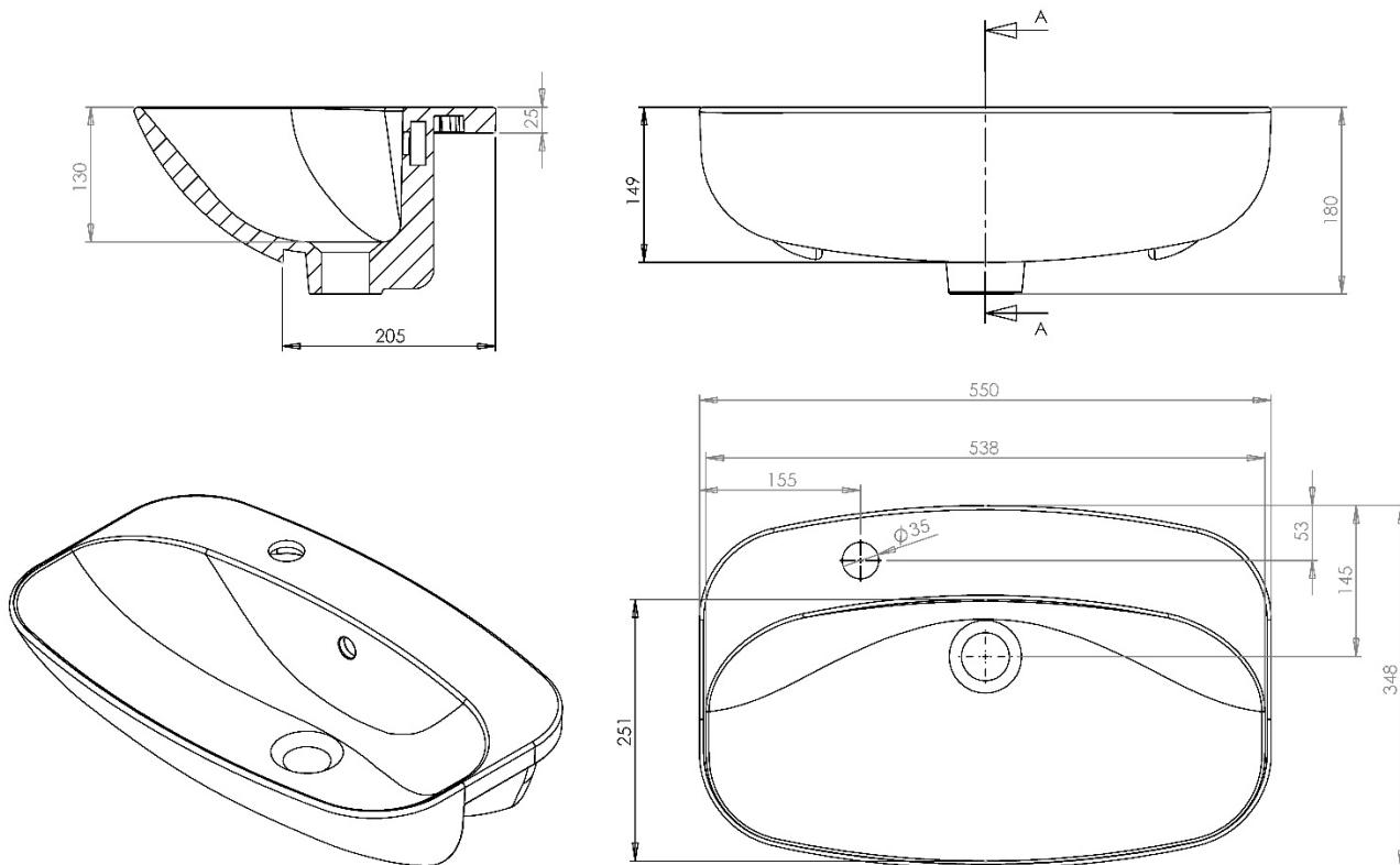
All dimension in mm. Please check dimensions prior to installation as they can vary due to manufacturing tolerances.
